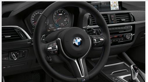
Depending on the equipment, Multifunction for steering wheel can be used to operate the telephone, voice control and audio functions via the buttons on the steering wheel. The Manual Speed Limiter is also integrated. It can be used to set an upper limit of 50 km/h for city driving, for example.
