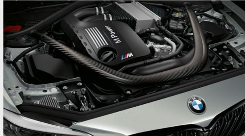
■ The front end strut brace made of carbon fibre reinforced plastic (CFRP) is a significant body component in the engine compartment that comes from motor-sport vehicles. Though it weighs only 1.5 kg, it significantly increases frontend rigidity and contributes to greater steering precision and accuracy.
