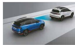
Forward Collision - Avoidance Assist - Car (FCA-Car) & Forward Collision Warning (FCW)
