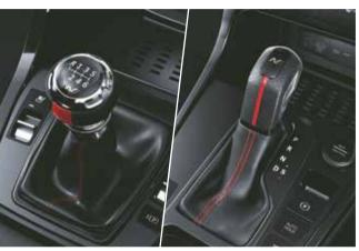
6-speed MT (Manual transmission) & 7-speed DCT (Dual clutch transmission)
