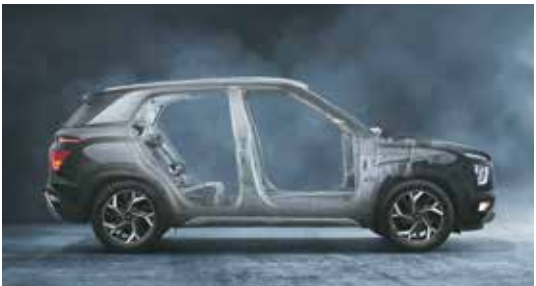
Strong body structure with AHSS
