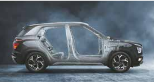
Strong Body Structure with AHSS
