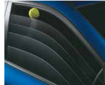
Auto Up/Down Power Window with Pinch Guard
