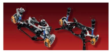
Handling duties are managed by a sophisticated 4-wheel independent suspension system mounted to high-precision 6-point front and rear subframes. A special Bilstein DampTronic driver adjustable shock absorber system utilizes multiple vehicle information systems to provide appropriate damping forces and a high level of control for a variety of driving situations.
