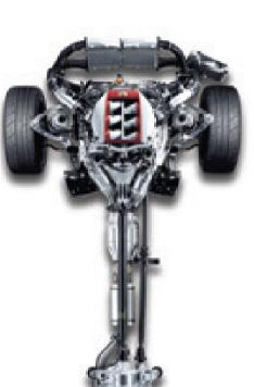
Dry Sump Lubrication System To ensure stable lubrication for the transmission even when cornering at high Gs, a dry sump lubrication system is employed. The system sprays transmission oil directly onto the gears. reducing friction and increasing reliability.
