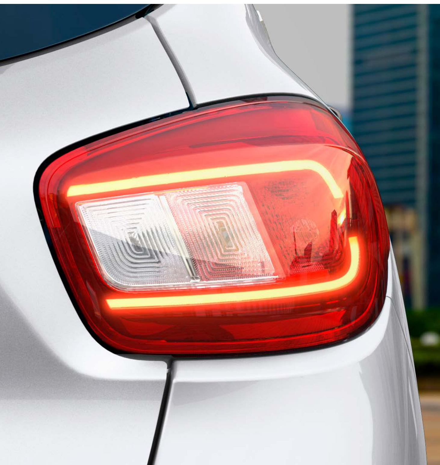
tail lamps with LED light guides
