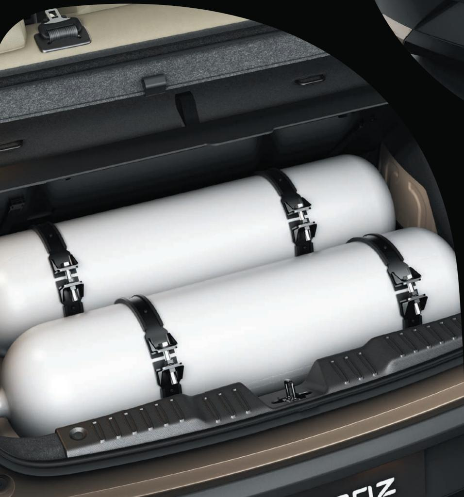
The twin CNG cylinders of 60 litres capacity are placed hidden beneath the luggage area for a high on aesthetics and unbelievably huge boot space. The advanced iCNG technology offers incredible petrol car like performance with an unmatched power of 73.5 PS and torque of 103 NM.
