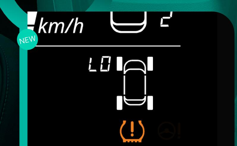
Tyre Pressure Monitoring System (Indirect)
