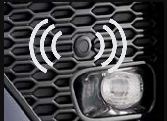
Front Clearance Sonar with MID Indication
