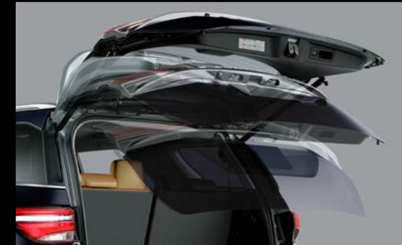
Electronically Controlled Power Back Door with Memory & Jam Protection
