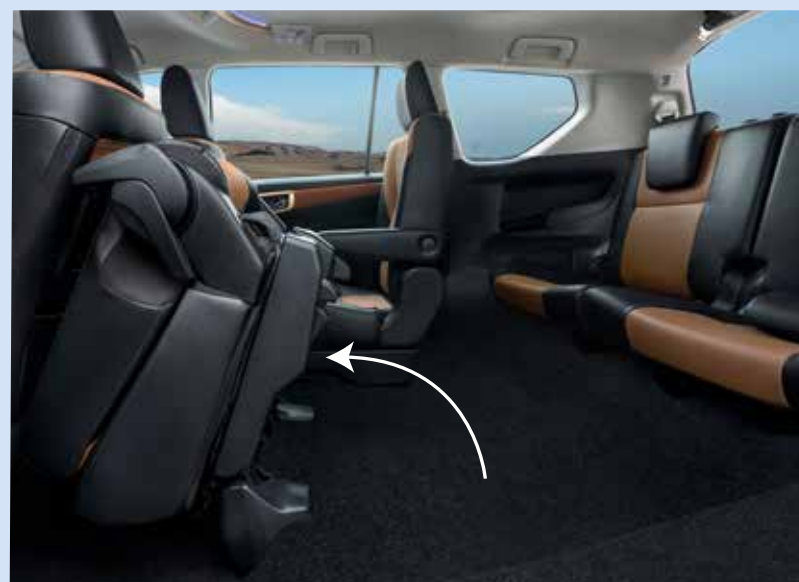
One-touch Tumble Second Row Seat Gives you easy access to the third row seats
