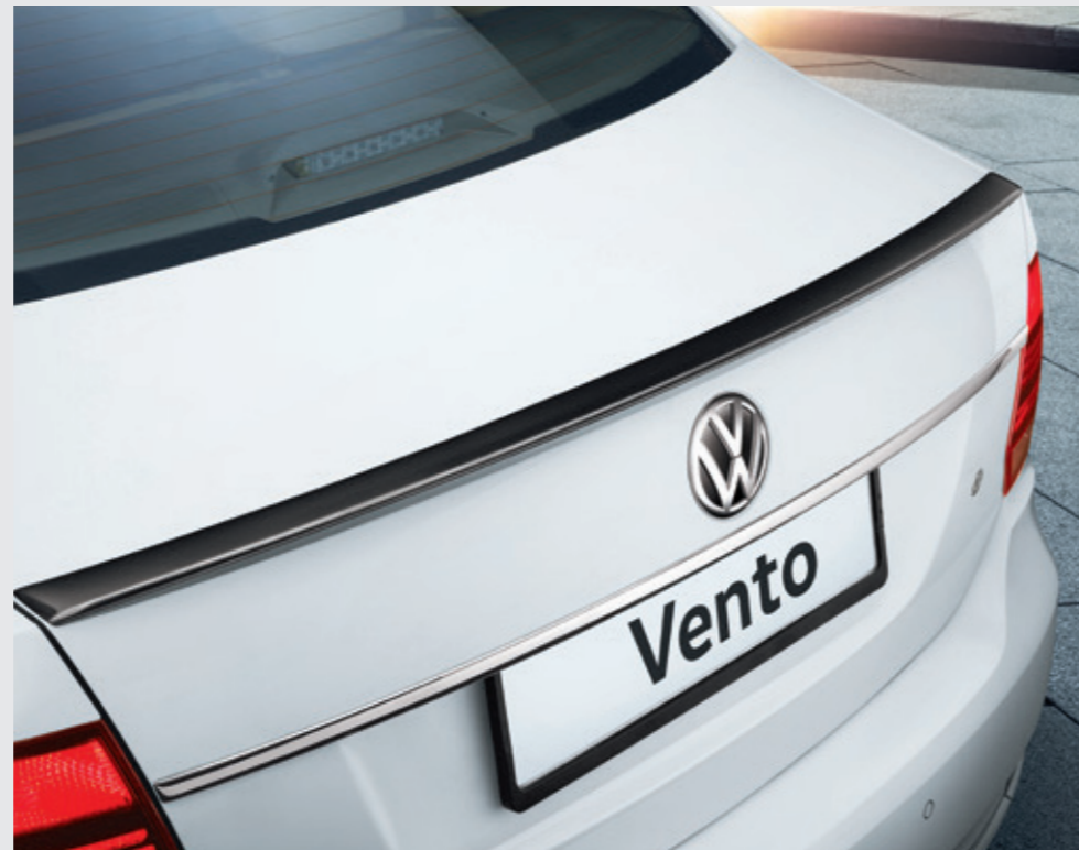
Trunk Lip Spoiler - Primed / Deep Black / Candy White / Reflex Silver Carbon Steel Grey / Titanium Beige Part No. 6RF071641GRU / 6RF071641C9X / 6RF071641B9A / 6RF071641A7W 6RF071641A9W / 6RF071641A1X
